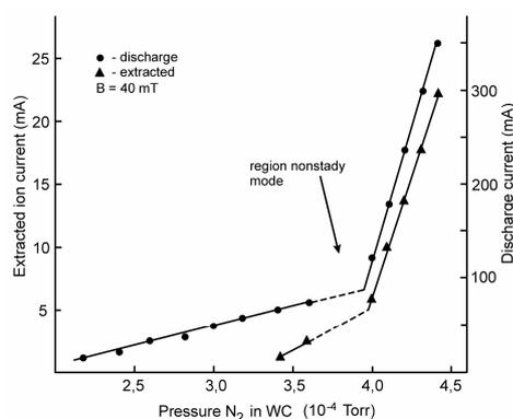
Fig. 4. Dependence discharge and extracted currents versus the working gas pressure
