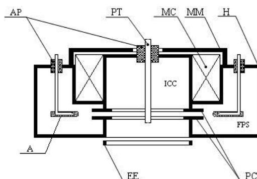
Fig. 1. A schematic diagram TIS of coaxial geometry: The source of the gas plasma FPS-I; the internal cylindrical chamber ICC-II of the TIS; A – the annular anode, PC – the cold poles-cathodes; MC – solenoid; MM – the maker for inverted flow of compound magnet; H – housing; PT – the axial isolated electrode the probe; EE – the extracting electrode,  $U_a$  – voltage of anode,  $U_i$  and  $U_e$  – voltages of the PT and of the EE relatively housing
