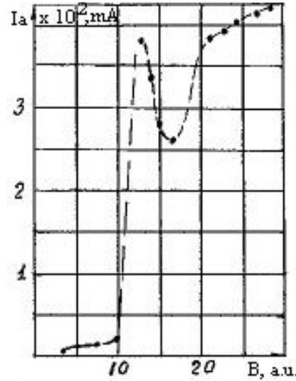
Fig. 6. The current of the LDC discharge as a function of induction  $B_a$  (of the Is) in spacing
