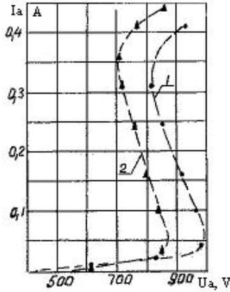
Fig. 5. Dependence discharge current versus of the anode voltage
