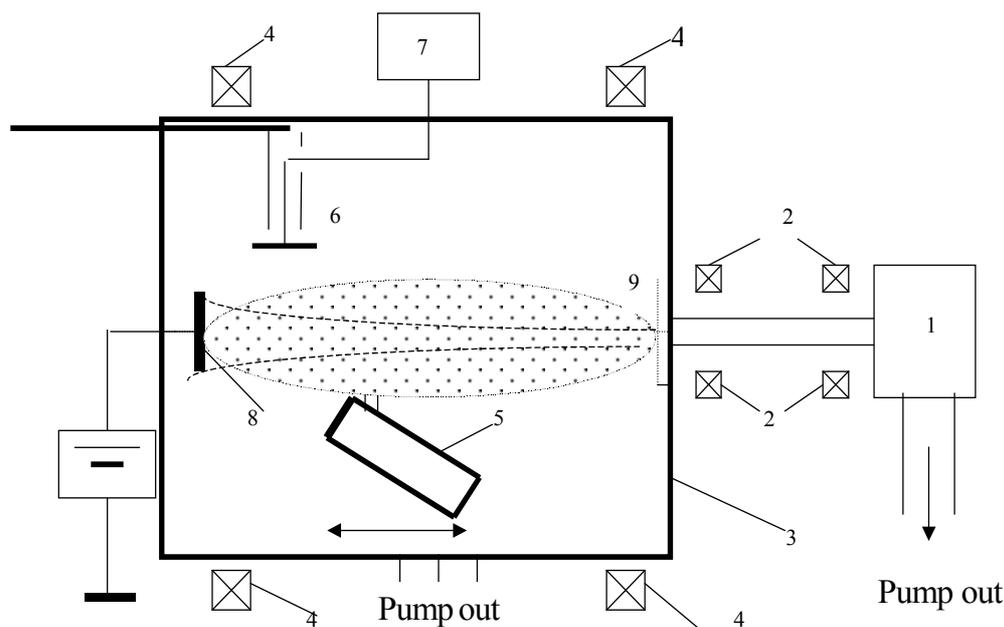
Fig. 1. An installation diagram. 1 – injector of electrons, 2 – focusing coils, 3 – evacuated chamber, 4 – Helmholtz coils, 5 – analyzer of energy of ions, 6 – header of a sample, 7 – sensor of ion current to a substrate, 8 – collector of discharge, 9 – UHF modulator of a beam
