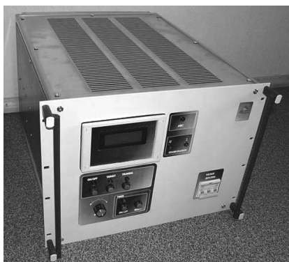
Fig. 5. External view of the pulsed voltage supply of electric substrate displacement
