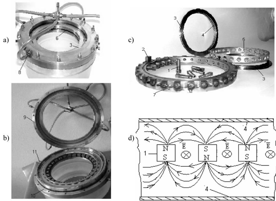
Fig. 1. The discharger: outward appearance (a), the basic constituents (b, c), and a sketch of crossed  $E \times H$  – fields (d)
