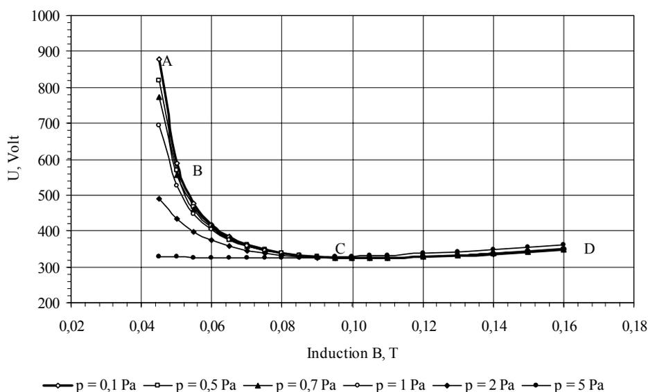
Fig. 3. Rated dependences  $U_{ign}=f(pdB_{\perp}/p)$ , where  $d=2$  mm
