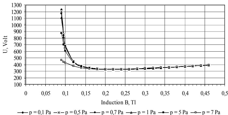
Fig. 2. Rated dependences  $U_{ign}=f(pdB_{\perp}/p)$ , where  $d=0,95$  mm
