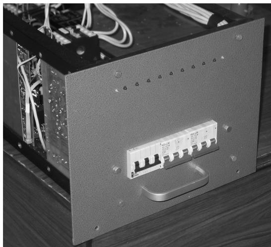
Fig. 3. Power supply unit of the automatic control system for the Raduga-5 source of accelerated metal ions
