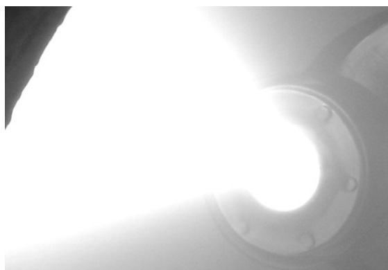
Fig. 5. The photo of hybrid magnetron-arc discharge
