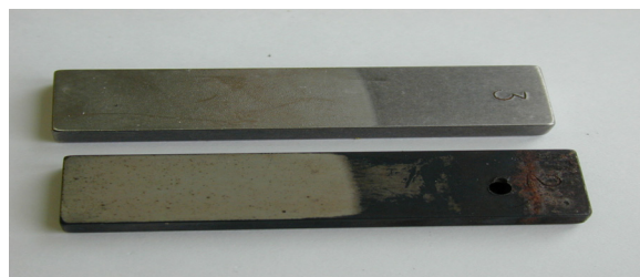
Fig. 1. Photograph of EP866sh steel specimens before and after corrosion tests under the thermocycling conditions ( T=600 \text{ }^\circ\text{C} , seawater at 20 °C, 20 cycles, irradiation with mask w=20\text{--}22 \text{ J/cm}^2 , n=5 pulses
