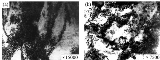
Fig. 3. Image of cellular structure of AMg6 alloy irradiated with  $\text{Ar}^+$  ions at  $E=20 \text{keV}$ ,  $j=150 \mu\text{A}/\text{cm}^2$ : a –  $D=10^{15} \text{cm}^{-2}$ ; b –  $D=10^{17} \text{cm}^{-2}$
