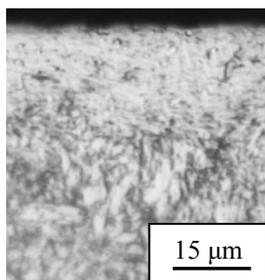
Fig. 1. Metallographic picture of the surface layer of steel 40X13 after ultrasonic modification
