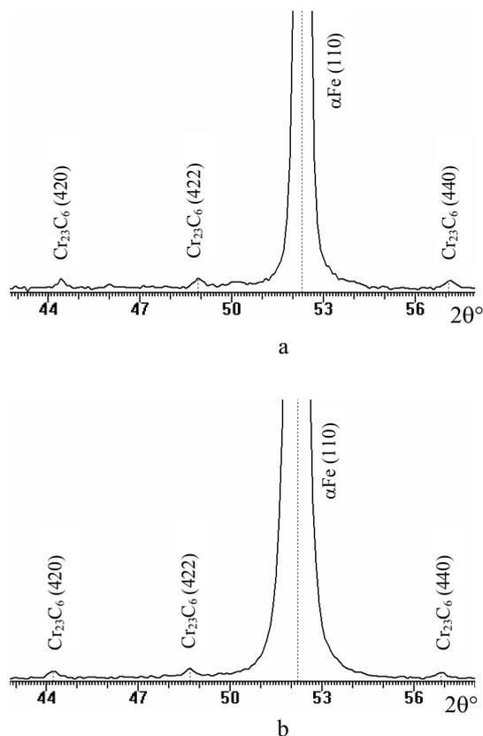
Fig. 2. Fragments of X-ray diffractograms ( $CoK_{\alpha}$ ) from the surface layers of steel 40X13: a – after grinding, b – after ultrasonic modification
