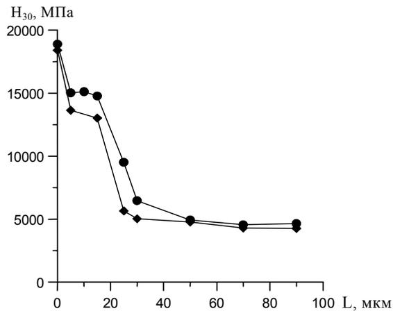
Fig. 5. Changes in microhardness values to the depth of the implanted layer at  $T=450$  °C:  $\blacklozenge$  – implantation N<sup>+</sup> after grinding,  $\bullet$  – implantation N<sup>+</sup> after ultrasonic treatment
