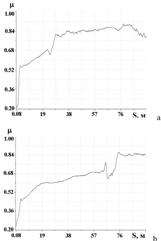
Fig. 6. Dependence of size of factor of friction on length of a way indenter on steel 40X13 with nitrated by a layer: a – after grinding, b – after ultrasonic modification
