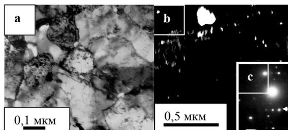
Fig. 3. Electron-microscopic images of structure of surface layers of steel 40X13 after ultrasonic modification: a – light field, b – dark field in the reflection  $[115] Cr_{23}C_6$ , c – microelectron diffraction
