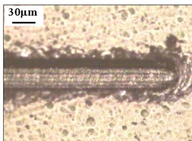
Fig. 5. The results of one experiment, where a coating hasn't been damaged during scratch-test (The loading rate 2 N/min). The film thickness is 1.6µm
