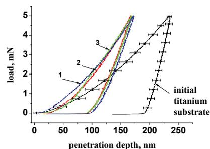
Fig. 4. Comparison between load-displacement curves for Ca-P coating and titanium substrate. The film thickness is  $1.6 \mu\text{m}$ . Curves 1, 2, 3 obtained for Ca-P coating
