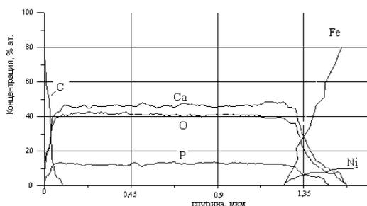
Fig. 3. The profiles of the elements distribution within the Ca-P coating on the 316L stainless steel substrate
