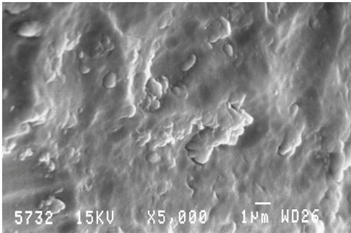
Fig. 1. The texture of the Ca-P coating on the titanium substrate. Magnification is 5000
