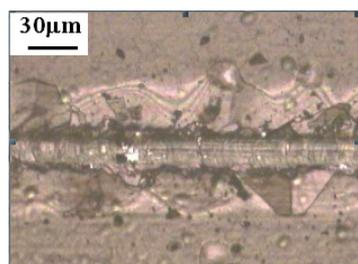
Fig. 6. The results of one experiment, where a coating has been damaged during scratch-test (photo was made at the loading rate 0.66 N/min). The film thickness is 2.7 µm
