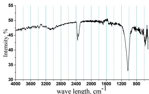
Fig. 2. The pattern of FTIR spectra of the Ca-P coating
