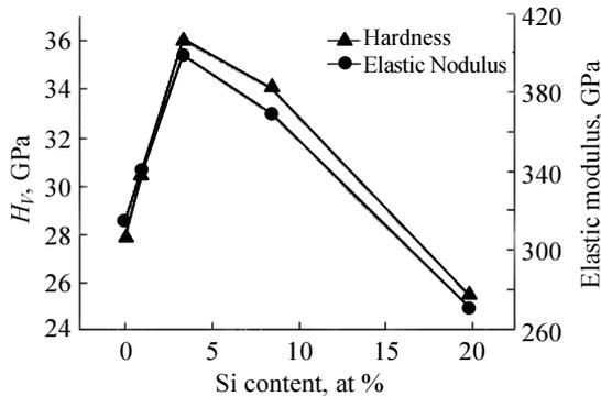
Fig. 2. Hardness and elastic modulus of the Ti-Al-Si-N films as a function of Si content [3]
