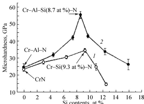
Fig. 9. Microhardness of the Cr-Si-N (1) and Cr-Al-Si-N (2) coatings as a function of Si content [13]
