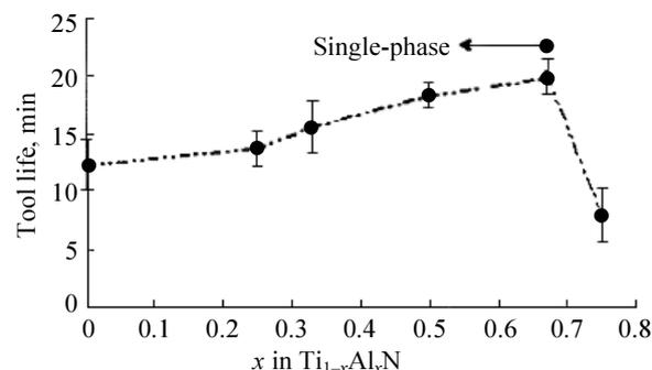
Fig. 1. Influence of Al content  $x$  in Ti<sub>1-x</sub>Al<sub>x</sub>N coatings on tool life at face milling tests [2]
