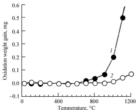
Fig. 6. Oxidation weight gain curves of TiAlN and (TiCrAl)N coating measured by thermo-balance [10]: 1 –  $(Ti_{0.5}Al_{0.5})N$ ; 2 –  $(Ti_{0.11}Cr_{0.2}Al_{0.69})N$
