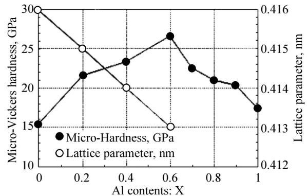
Fig. 5. Changes in micro-Vickers hardness and lattice parameter of Cr<sub>1-x</sub>Al<sub>x</sub>N films [9]
