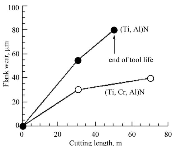
Fig. 7. Result of high-speed milling test against hardened die-steel in comparison with conventional TiAlN coatings [10]
