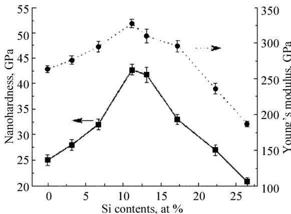
Fig. 4. Nanohardness and Young's modulus of Ti-Si-N coatings as a function of Si contents for an indentation load of 5 mN [5]
