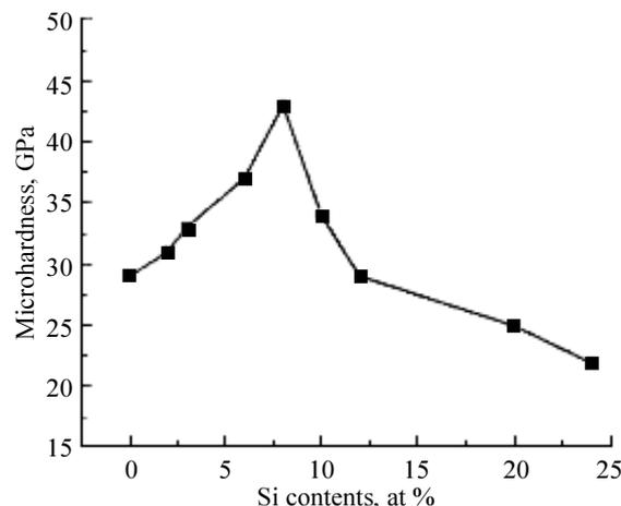
Fig. 10. Microhardness values of the Ti-Cr-Si-N coatings with various Si contents [14]
