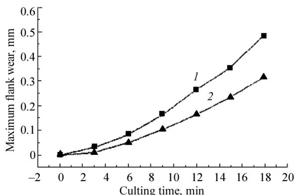
Fig. 8. The progress of flank wear measurements for  $(Ti_{0.34}Al_{0.66})N$  (1) and  $(Cr_{0.28}Al_{0.72})N$  (2) coatings by coatings by continuous turning of stainless steel with CNMG120408 style insert [12]
