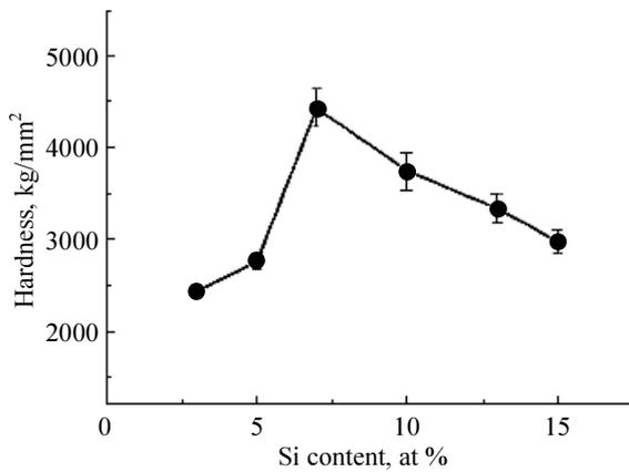
Fig. 3. Microhardness values of Ti-Si-N coating layers as a function of Si content [4]
