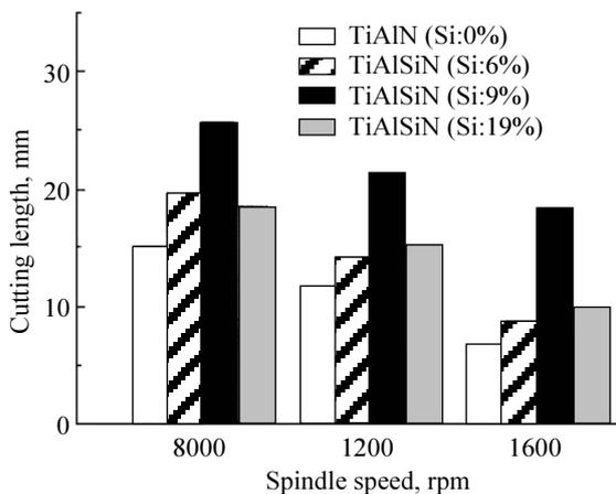
Fig. 12. The comparison of tool life according to Si contents in a series of spindle speed (8000, 12 000, 16 000 rpm) [18]
