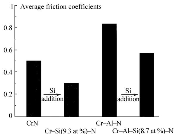
Fig. 11. Average friction coefficients of CrN, Cr-Si (9.3 at %)-N, Cr-Al-N, and Cr-Al-Si (8.7 at %)-N coatings against steel ball [13]
