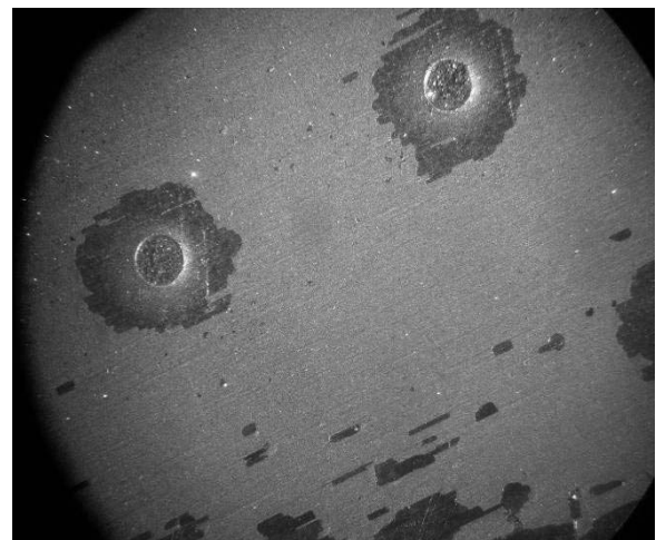
Fig. 2. Surface of electro arc coating \text{TiC}:\text{MoS}_x on the base made of steel ShH-15 without binding (adhesion) underlayer
