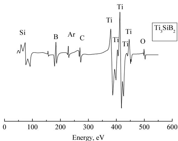
Fig. 4. Auger spectrum stated from samples surface with titanium-silicon-boron system coating
