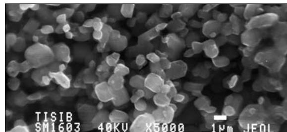
Fig. 1. Microstructure of cathode material, made by SHS method (TiB<sub>2</sub>, Ti<sub>5</sub>Si<sub>3</sub>, Ti<sub>3</sub>SiB<sub>2</sub>)
