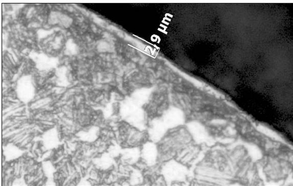
Fig. 2. Material microstructure in blade surface layer from alloy VT6 with Ti-Si-B coating
