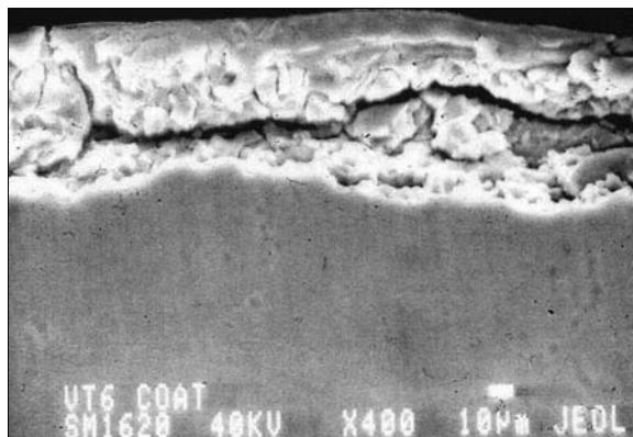
Fig. 5. SEM image of surface layer of sample with 6  $\mu\text{m}$  coating after accomplishment of fatigue tests
