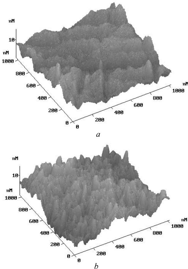
Fig. 3. AFM image of the SS surface without DLC film (a) ( $R_a = 1.9$  nm,  $R_q = 2.4$  nm) and with DLC film (b) ( $U_{bias} = -15$  kV) ( $R_a = 2.0$  nm,  $R_q = 2.5$  nm)
