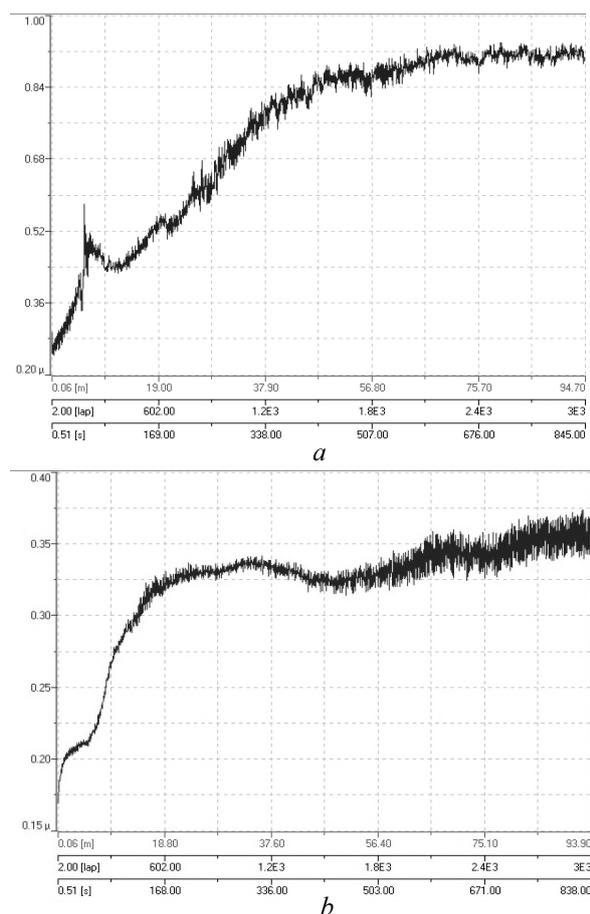
Fig. 2. Friction coefficient of the SS specimen without (a) and with DLC films (b)
