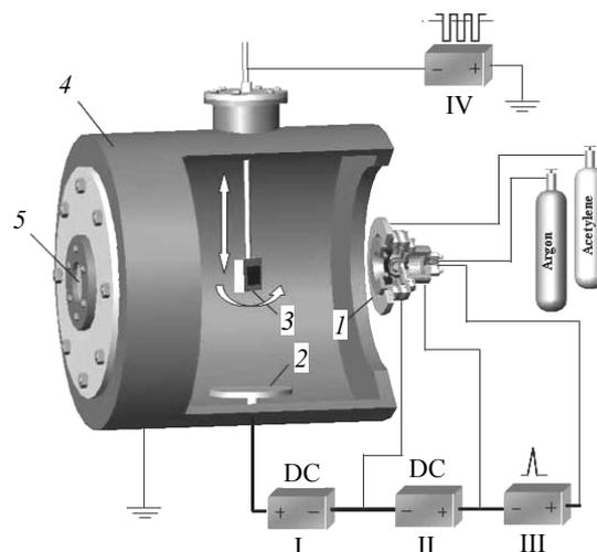
Fig. 1. Scheme of experimental setup: 1 – plasma generator; 2 – main discharge anode; 3 – moveable holder with specimen; 4 – vacuum chamber; 5 – window. Power supplies: I – main discharge; II – emitter discharge; III – trigger discharge; IV – pulse bias
