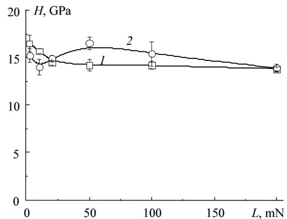
Fig. 4. Hardness versus nanoindenter load for the implanted specimens with DLC films. Amplitude of negative bias voltage in DLC film deposition: 1 – 10; 2 – 15 kV
