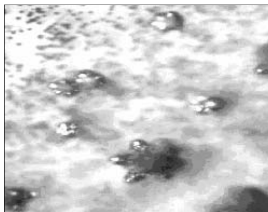
Fig. 2. Nickel release from pores of a track template on the surface of TM, K = 10000
