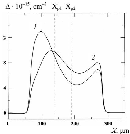
Fig. 3. Distributions of the accumulated plasma concentration at  $t^+ = 2 \mu\text{s}$ ,  $S_{\text{SOS}} = 4 \text{ cm}^2$  across the structure having  $X_p = 140 \mu\text{m}$  (curve 1) and  $X_p = 190 \mu\text{m}$  (curve 2)
